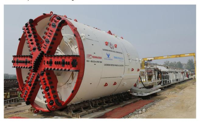
Two 6.52m diameter TERRATEC Earth Pressure Balance (EPB) Tunnel Boring Machines are ready to be delivered to Tata-Gulermak JV, for the North-South line (Phase 1 A) of the Lucknow Metro, in Uttar Pradesh, India.
